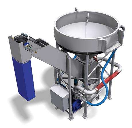
Our Cyclone Destoner gently separates stones from produce, particularly carrots. Produce and stones are fed into a moving well of water in the Cyclone Destoner cone. Produce stays near the water surface and exits via an outfeed flume.
