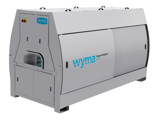
Our Vege-Polisher™ has a rotating drum made up of rows of nylon brushes. Produce enters via a large infeed chute. Two water pipes spray fresh and/or recycled water on the produce as it travels through the drum. Produce is washed/polished as it rubs against other produce as well as the rotating brushes. At the outfeed, produce slides down a chute with minimal drop for a smooth transition to downstream equipment.
