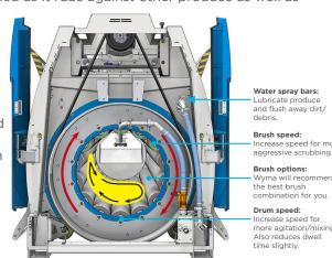
Water spray bars: Lubricate produce and flush away dirt/debris.
