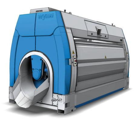
Our Vege-Polisher™ has a rotating drum made up of rows of nylon brushes. Produce enters via a large in-feed chute. Two water pipes spray fresh and/or recycled water on the produce as it travels through the drum. Produce is washed/polished as it rubs against other produce as well as the rotating brushes.
