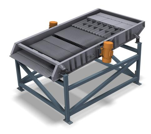
Produce is fed onto a flat section at the infeed end of the machine (spreader tray). It then moves onto the bed which is made up of corrugated channels. The whole machine vibrates and spreads produce across its width. The vibrations also move produce into the corrugated channels and towards the outfeed.
